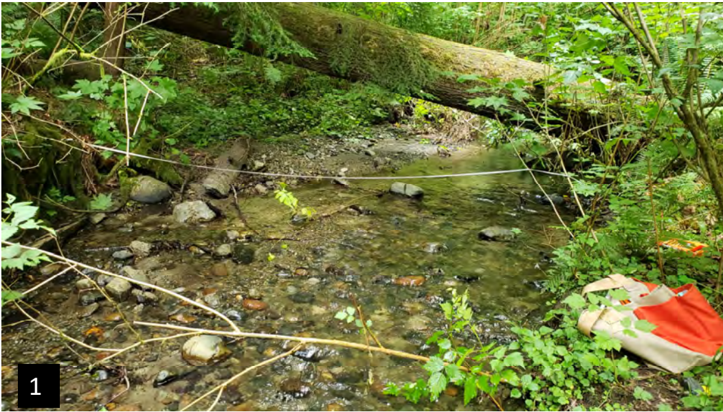
~620 ft upstream of culvert BFW measurement #1 = 13 ft Wolman pebble count #1
